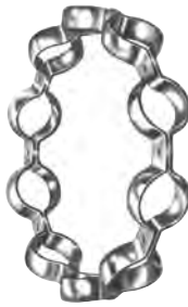
Fig. A-2. Pressed-steel welded cage.
