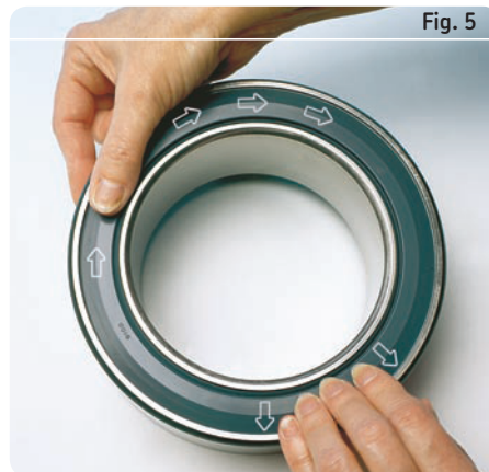
Inserting the seal in the outer ring
