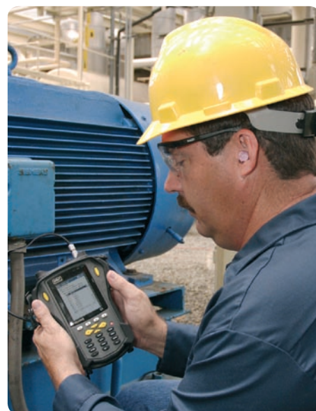
Recording vibration values using a SKF Microlog data collector
